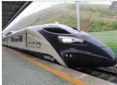
HEMU-430X High-speed train with a world-class maximum test speed of 430 km/h
